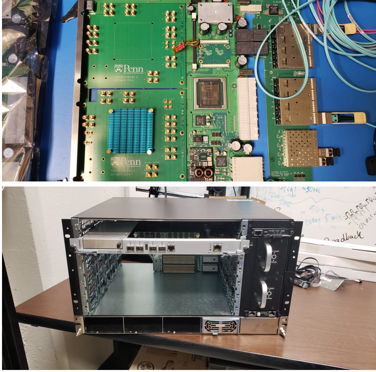
Figure 4.4: Top: an HTT demonstrator blade. Two TFM demonstrators are present, one with a heat sink installed, the other empty. The back of the blade is on the right, containing the connectors that insert into the shelf. The main processing FPGA is seen installed near the center, while the connectors for the management SoC are seen just above it. The IPMC is inserted into the long vertical black connector to the left of the SoC slot. Bottom: the blade inserted in to an ATCA crate.
