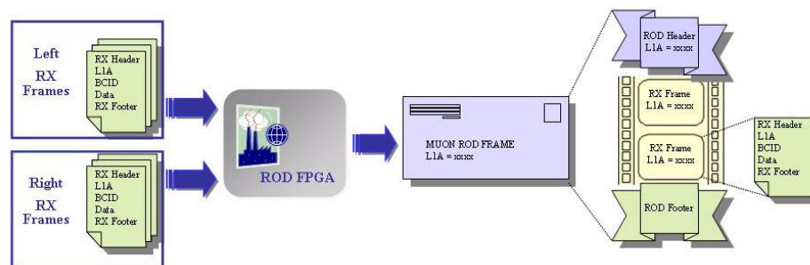
Fig. 3.7 The working principle scheme of the ROD "event builder"
