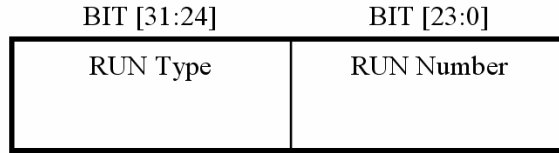
Fig. A.15 The Run_Number_config register
