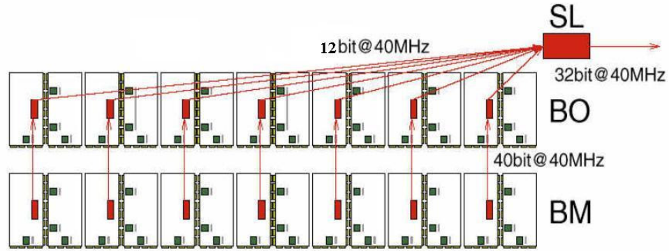
Fig. 2.34 The trigger information path from a “ Small ”sector to a SL
