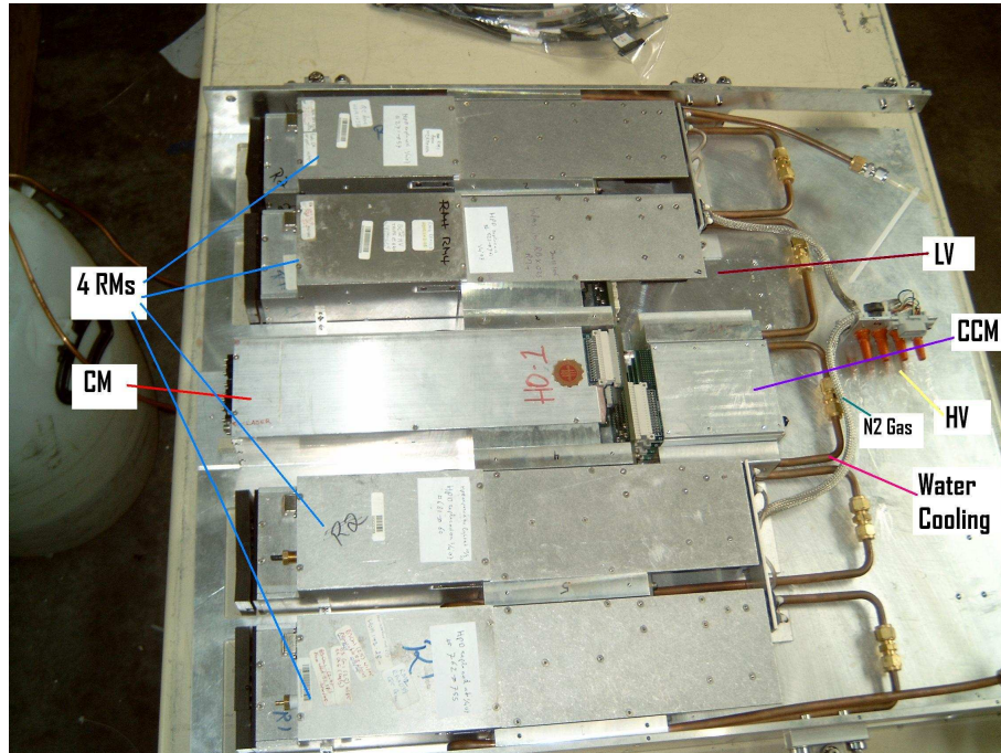
Figure 4.27: Complete RBX with 4 RMs, calibration module, CCM, and HV and LV supply link.
