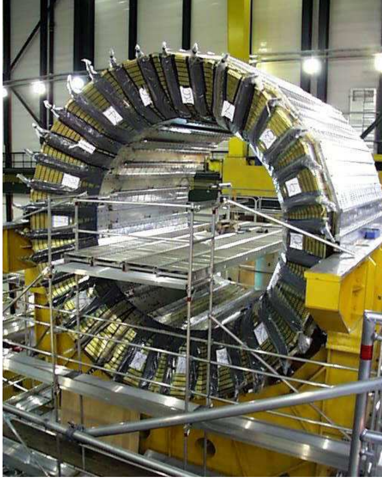
Figure 3.4: Assembled hadron barral (HB) before final installation in to the CMS detector.
