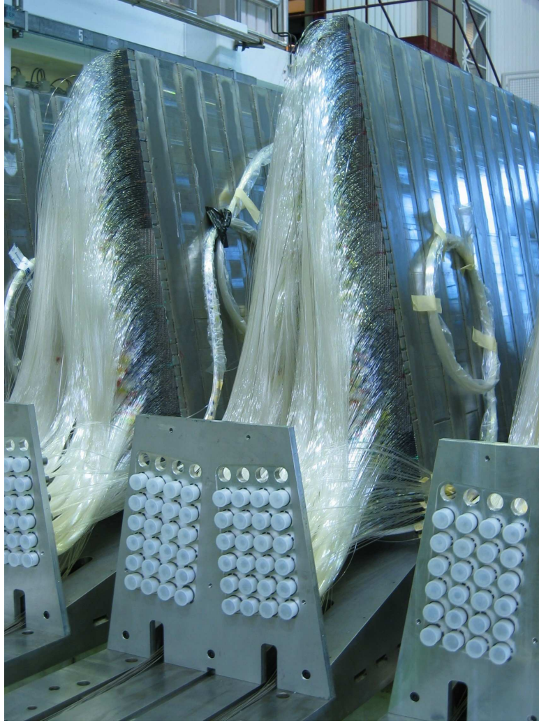
Figure 3.5: Hadron forward detector wedges with quartz fibers as sensitive detectors .
