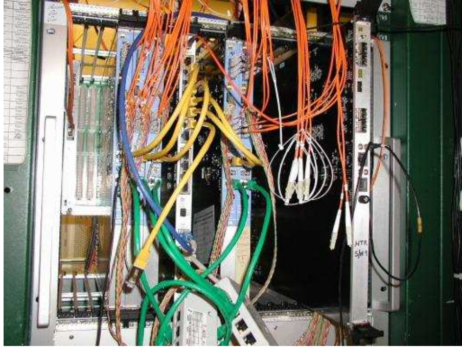
Figure 4.26: The readout crate with 6 HTRs, one trigger timing and control (TTC), a Fan Out, and a data concentrator card (DCC).
