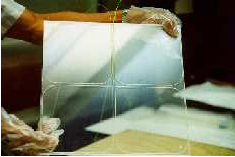
Figure 3.7: Picture of scintillator tray after machining
