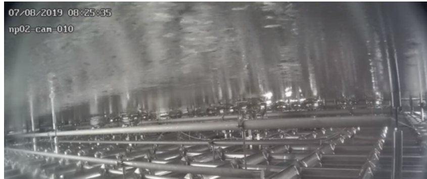
FIGURE 6.9: Picture taken with the cryogenic camera pointing to the PMT array taken on the 8 th of July 2019. The LAr level had just completely covered the PMTs.
