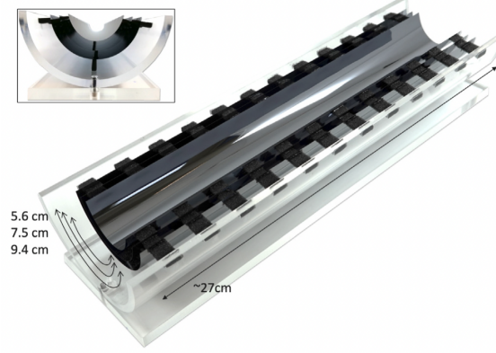
Figure 2.7: Installation model of all three layers of ALICE ITS3 [15]
