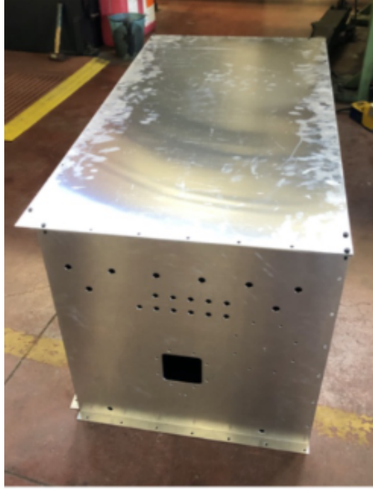
Figure 3.7. Faraday cage of aluminium
