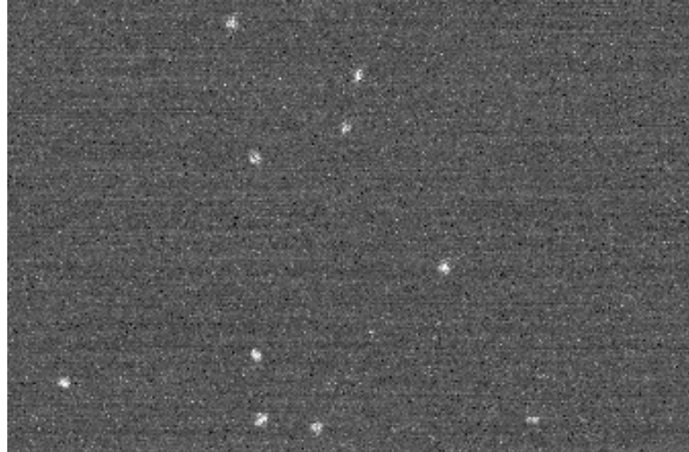
Figure 3.8. Light spots produced by the electronic cloud when it reaches the GEMs. The electronic cloud is composed by primary electrons produced by the interaction between the photo-electron and the gas atoms or molecules.
