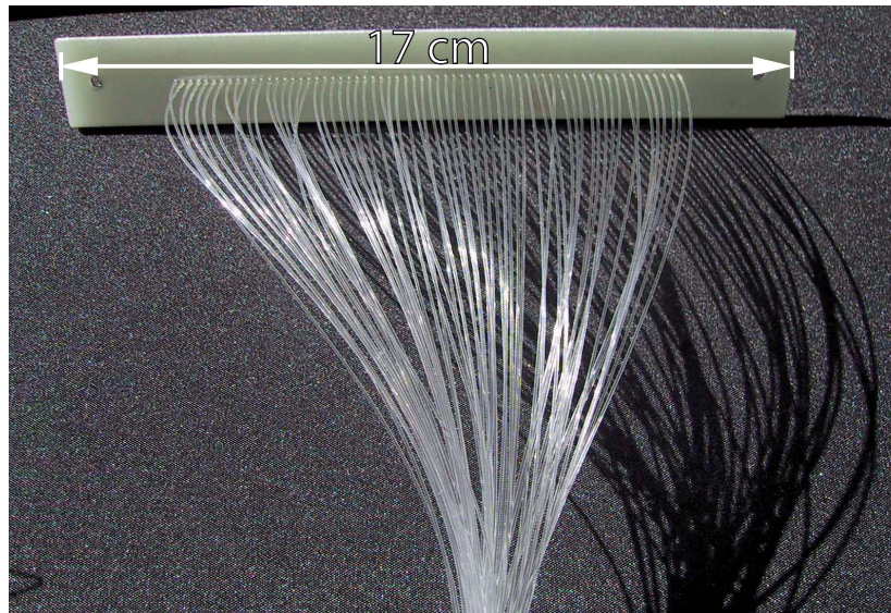
Figure 3.6: The fibres end in an array which is placed on top of a sensor. Because of the sequence of the fibres only one led spot is seen on an APV when single LEDs are switched on.
