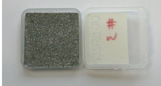
Figure 4.3: The sample powder is attached to the bottom of a plastic box [103]. The box can be closed for safer storage and opened for measurements.
