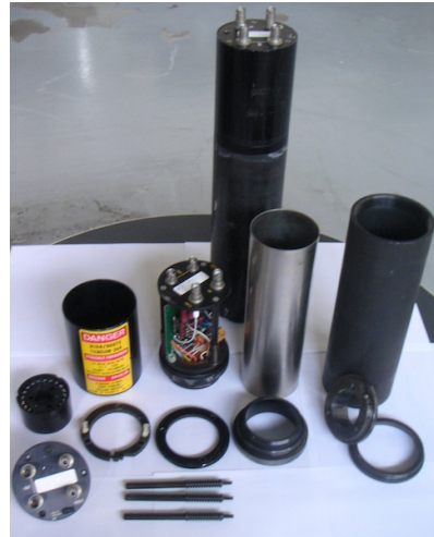
Figure 6.6: An R1828-01 PMT [125] (left) and the disassembled components of a PMT housing with an assembled housing at the rear (right). The device with internal wiring visible and external coaxial connectors is the custom divider.
