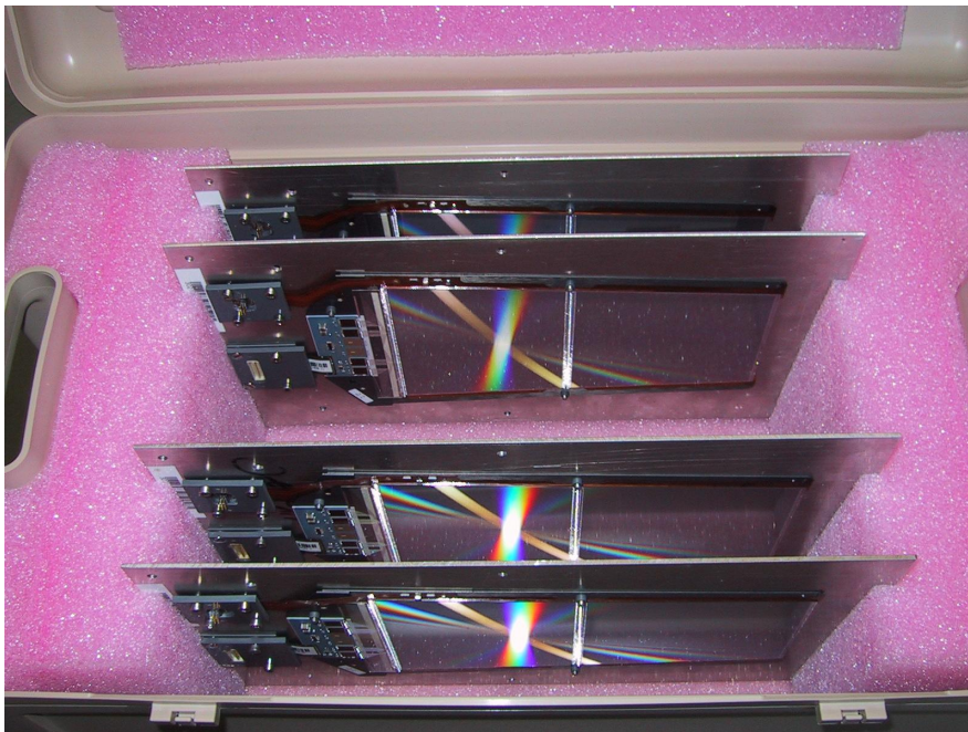
Figure 7.1: Transport box suited to hold up to ten modules mounted on their carrier plates.
