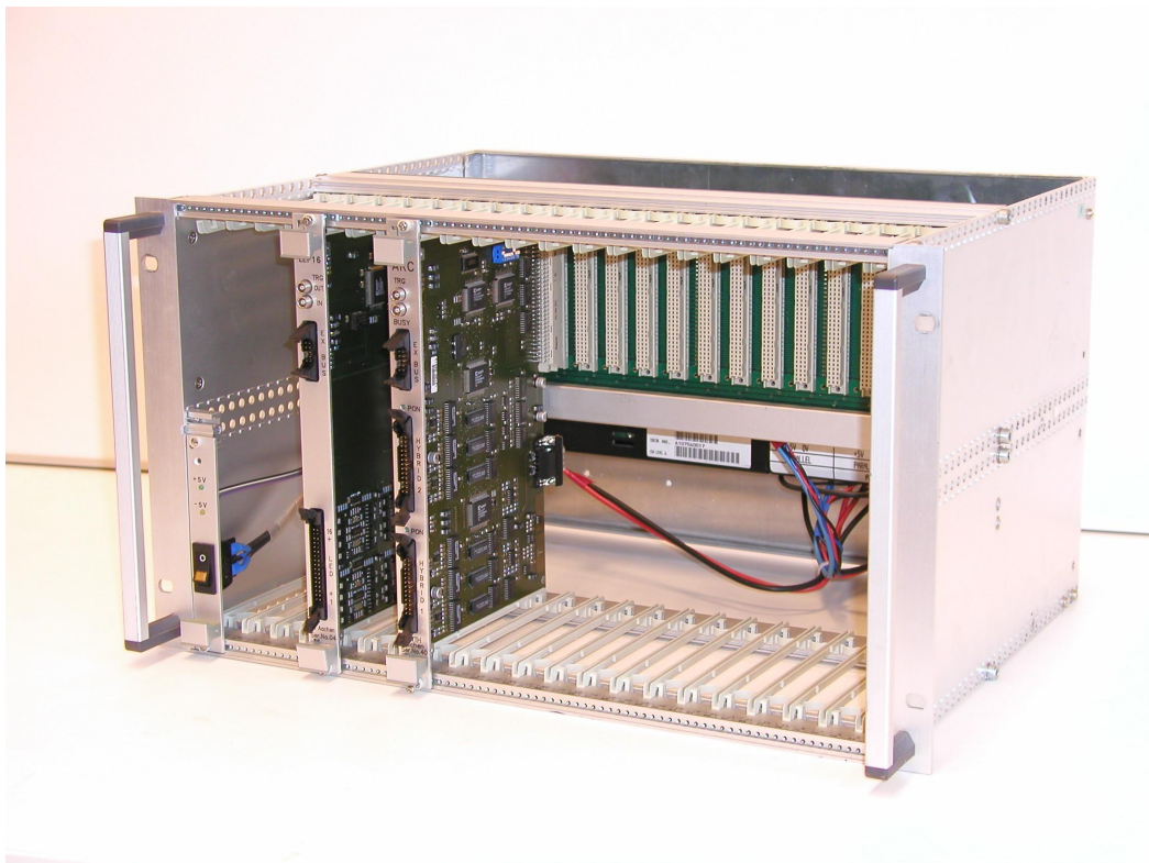
Figure 5.10: Crate equipped with one ARC board and one LED controller.
