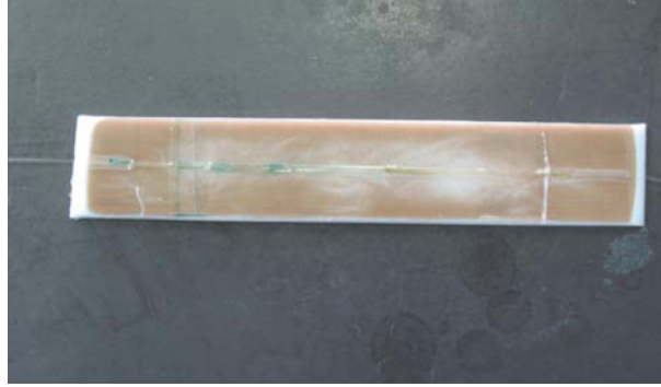
Figure 3.3: FBG bonded on a Teflon sample.
