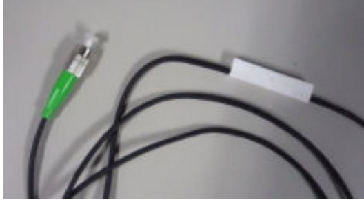
Figure 2.1: FBG sensor packaged with a ceramic material.
