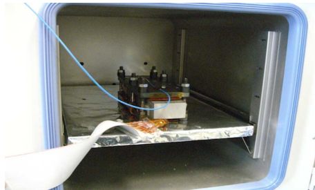
(f) Curing process at 90°C.
