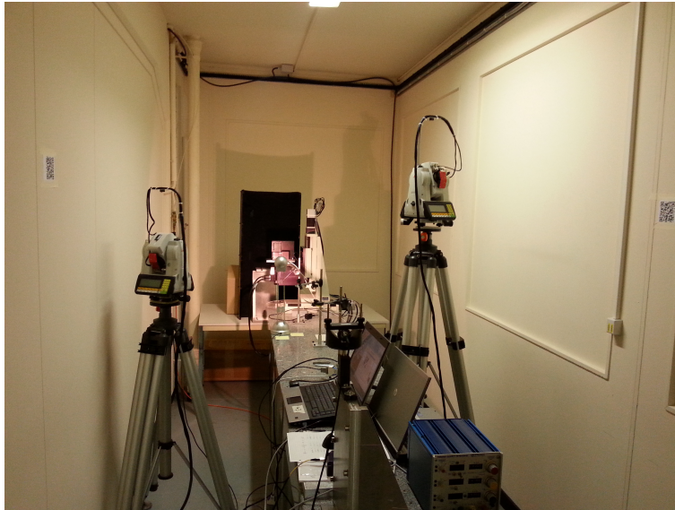
Figure F.4: Measurement bench in the optical lab and theodolites used for experiments of repositioning.
