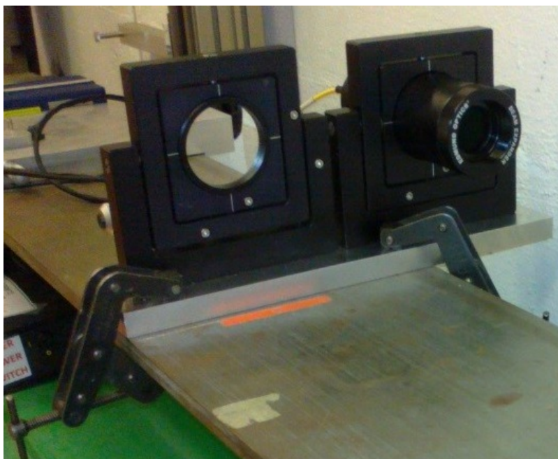
(a) One mirror (left) and beam expander (right) at one end of the rail.
