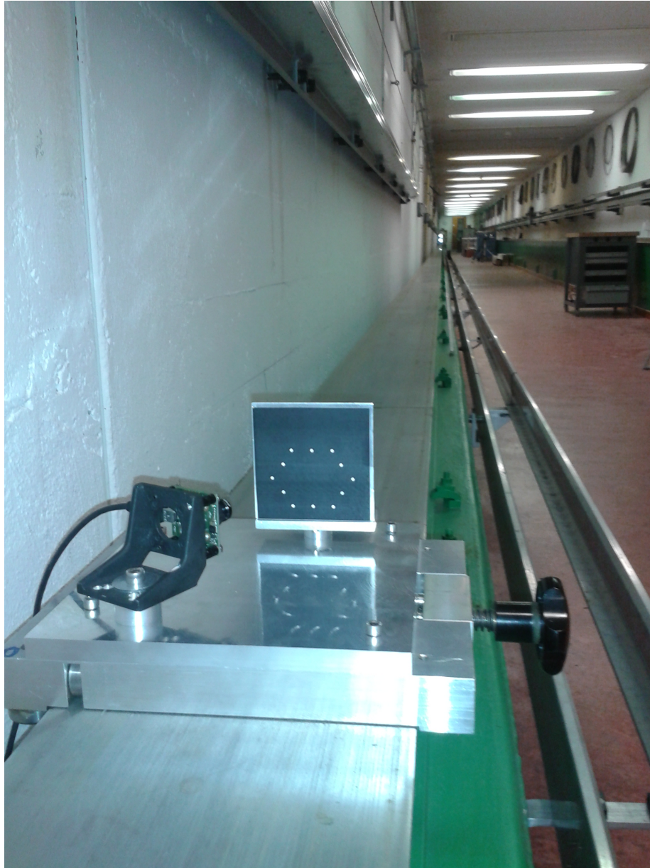
Figure F.5: Measurement bench used for long distance measurement in the geodetic base. The LAMBDA sensor can be manually displaced along a 50 m rail.
