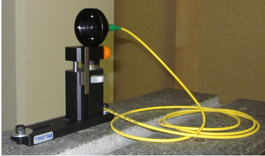
Figure F.12: Collimator and optical fibre used in combination with the lasers (F.6 and F.10) in order to have parallel beams over 3 m.
