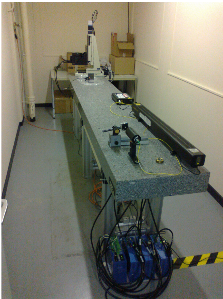
Figure F.2: Measurement bench used during 2013-2015 in the optical lab. Compared to the previous measurement bench (F.1), it is located in a closed room, which is better in terms of stability.
