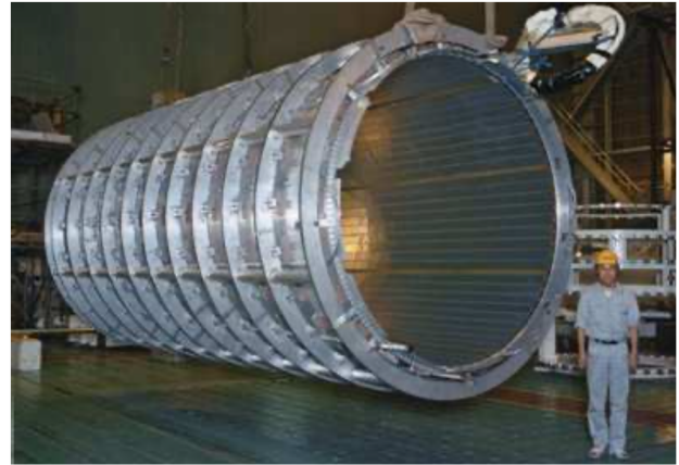
Figure 2.9: Picture of the solenoid after the completion of the wire envelope [2].
