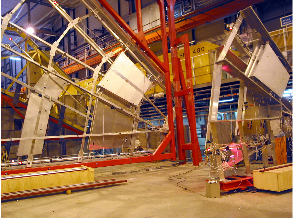
Figure 8.2: Picture of the three octants of the H8 test stand; (from left to right: EO-layer, EM-layer, EI-layer). The six alignment bars in this setup are marked with a red circle.
