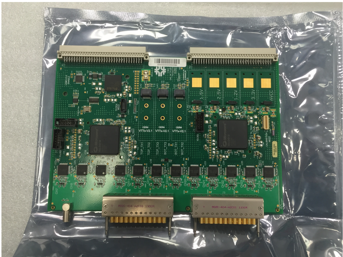
Figure 7.2. QIE card without VTTxs, DC-DC converters and front plates.
