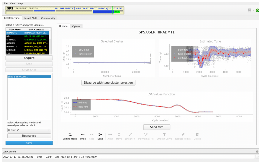
Figure 3.19: SPS Tune app: Betatron Tune analysis for the HIRADMT1 timing user for the horizontal plane.
