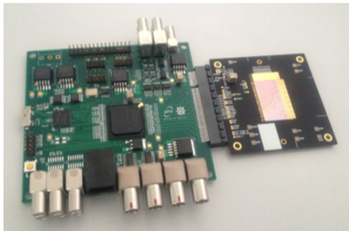
Figure 2.13 – DAQ read-out board connected an ALPIDE chip
