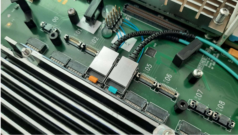
Figure 5.1: A Firefly transmitter (orange label) and receiver (blue label) pair connected to a Serenity board. When in use, a heat sink is mounted on top of the transceivers to maintain a low operating temperature to avoid damage to the parts. The FPGA is covered by the heat sink in the bottom left corner.
