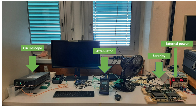
Figure 5.21: The setup of a Serenity board with Firefly transceivers connected in a loopback via an attenuator. The picture also shows the optical oscilloscope and the external power source.
