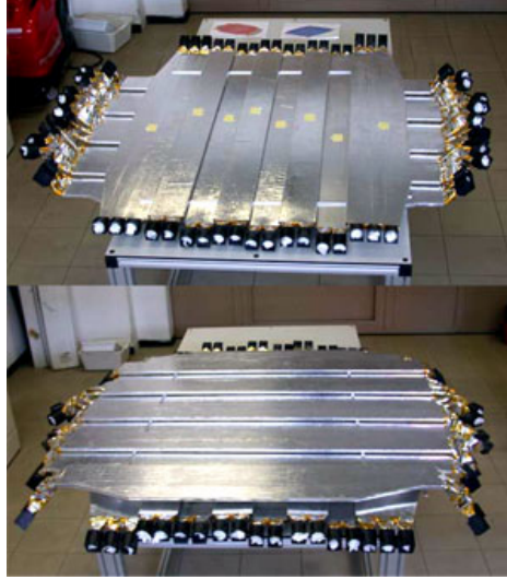
Figure 3.6.: The upper and lower part of the Time-of-Flight detector before integration. The velocity of the particle is measured by the difference of the time measurement of the single layers. [121]
