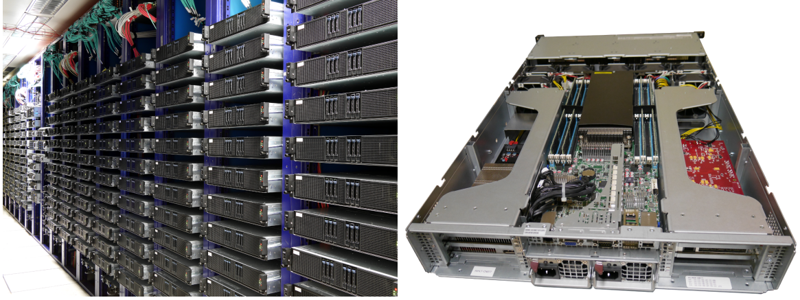
Figure 3.2: Left: Photo of the ALICE HLT at start of RUN 2. Right: interior of a node. The GPU is installed in the left tray, the C-RORC in red on the right.
