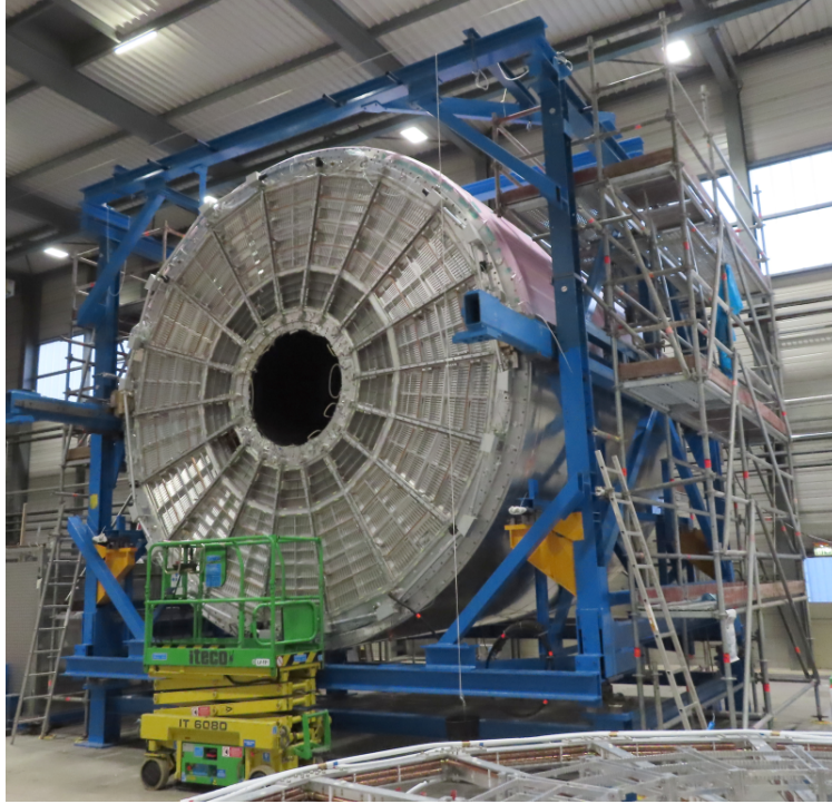
Figure 2.7: Photograph of the TPC, when it had been taken out from the ALICE cavern for the upgrade.
