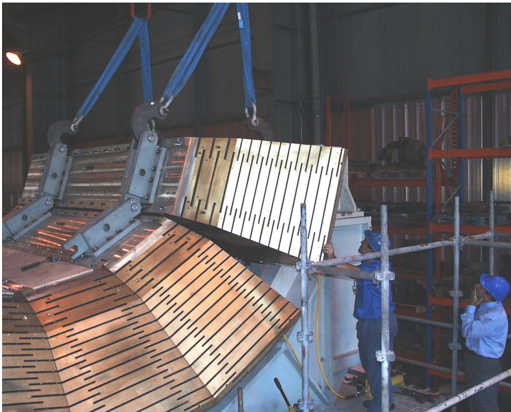
Figure 4.13: Assembling of the hadronic calorimeter brass wedge. Plastic scintillators are inserted between the brass plates ( Brice, Vaillet, and Lazic, 2008 ).
