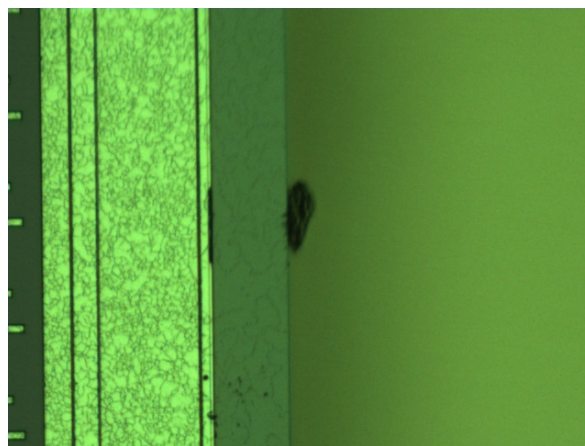
Figure 7.9: Photo recorded during the EI of the edge of sensor 35958_015_2-S_MAIN0 taken with the help of the LV program. A chip at the edge can be observed.
