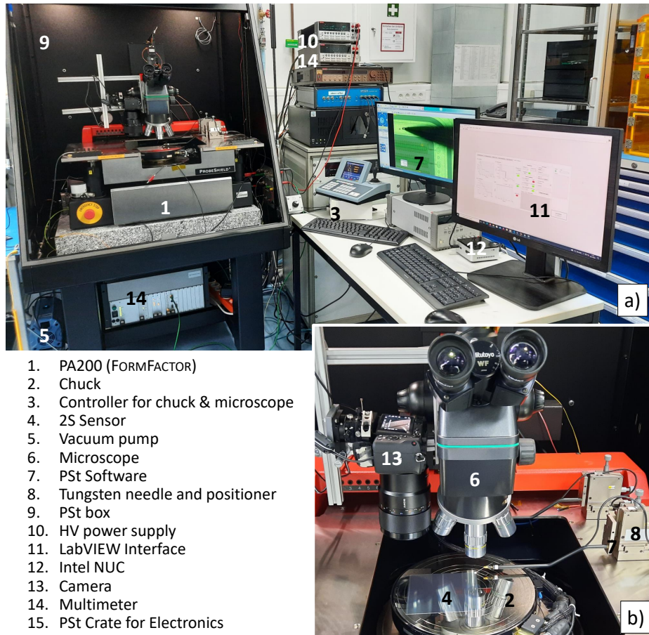
Figure 4.1: a) The Probe station test stand with associated components and b) a closer look to the centre of the test stand.
