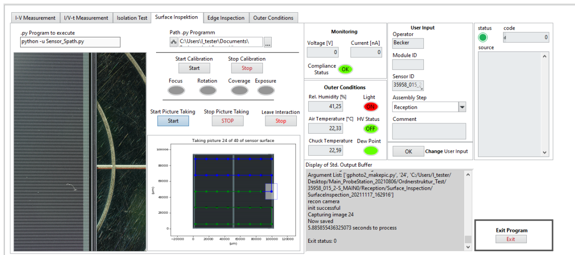
Figure 7.6: Screenshot of the front panel during the SI of sensor 35958.015.2-S.MAIN0.
