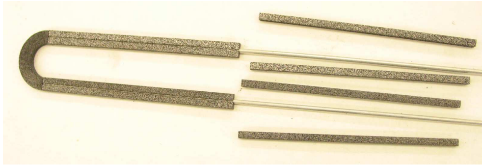
Figure 1.7: The round aluminium tube surrounding by PocoFaom pieces
