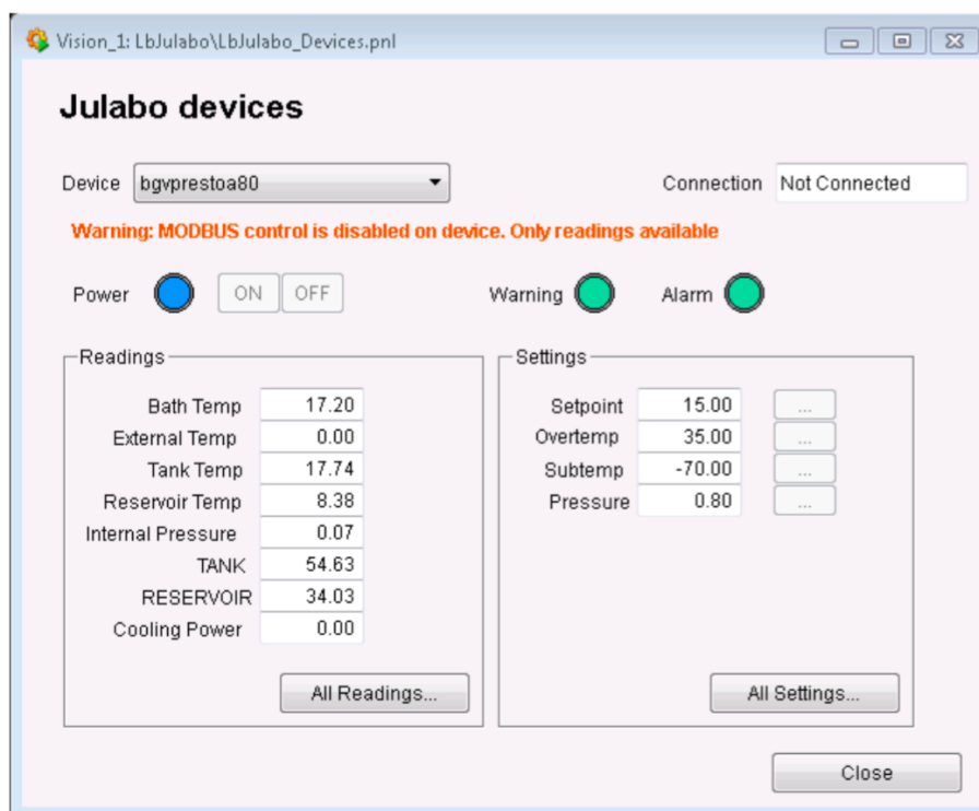
Figure 3.41: Control panel of the chiller. The panel displays several adjustable parameters of the chiller such as pressure [bar] and temperatures setpoint [°C]. Courtesy of L. Granado Cardoso.
