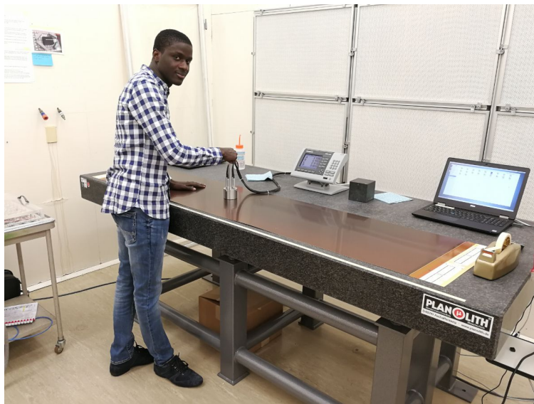
FIGURE E.3: Taking shift at CERN building 188, this step corresponds to the pillar heights measurement.
