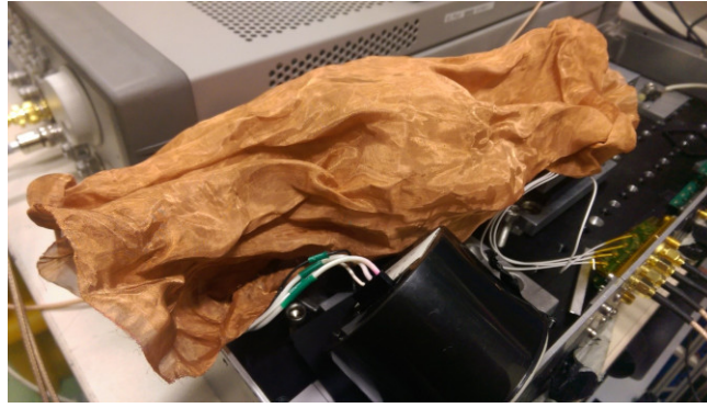
Figure B.3: The fine copper mesh used for the shielding experiments plotted in Figure 4.15.
