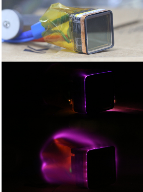
Figure 4.46: A corona produced during the vacuum tests of the PMT high voltage insulation. For safety of the device, all the PMT stages were grounded. At the top, a thin copper sheet can be seen wrapped around the PMT body near its front face, mostly covered with kapton insulation extending well beyond the PMT back side. In the middle and bottom images, a corona is forming with the decreasing pressure in the chamber as the copper sheet is biased at high voltage. The shape of the corona shows how the electric field lines are forced around the kapton insulation to reach the ground pins, proving the insulation at the front face of the PMT works as intended – no corona is seen anywhere at the PMT front face despite a much shorter path to ground than around the kapton insulation.
