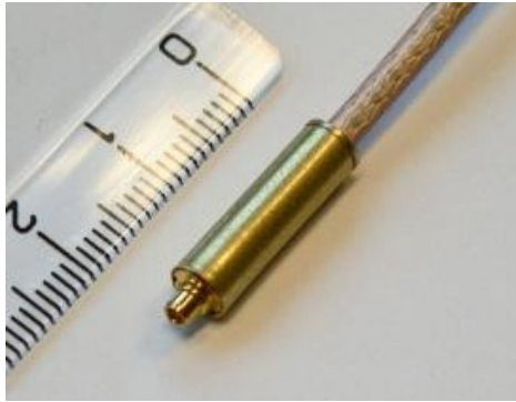
Figure 4.57: The new inline PAa. The MMCX connector plugs directly into its counterpart on the new PMT backend design, as described in section 4.6.
