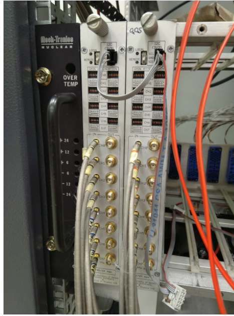
Figure 4.59: A pair of PAbc NIM modules. Note the change to MMCX connectors at the input and the I 2 C connection at the top.
