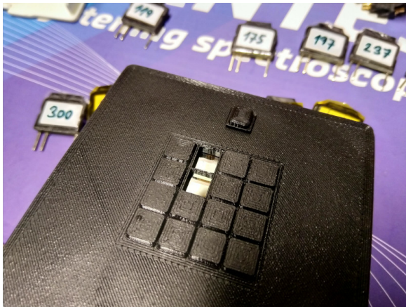
Figure 4.4: The 3D printed mask, a detail with a channel plug shown and in a mounted position during measurements of a single channel illumination scenario.
