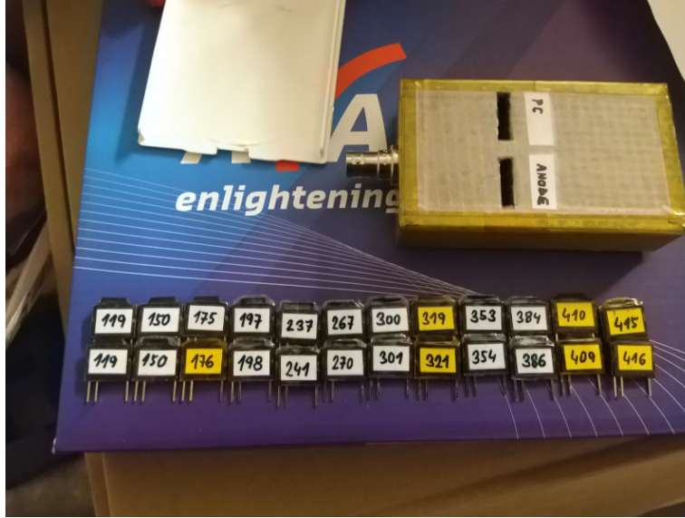
Figure 4.50: The experimental HV divider with the set of interchangeable modules laid out. The modules are inserted in the “PC” and “Anode” marked slots to determine the bias values at the front and back PMT stages. The MCP bias can be determined by subtracting these from the total bias.
