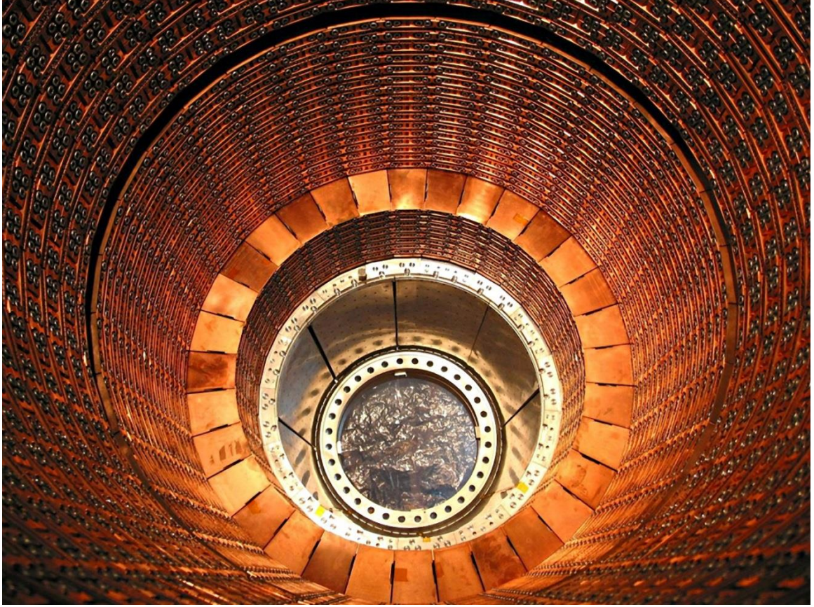
Figure 4: A view inside ATLAS's Electromagnetic Calorimeter. From [14].
