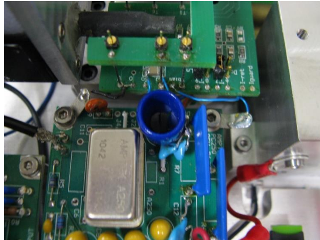
Figure 22: The plastic cup made to hold dry ice powder, currently empty. The FET can be seen inside the cup.
