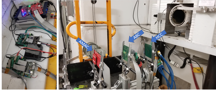
Figure 4.7: Photos of the setup for the two rounds of proton irradiation. LEFT: the FPGA arrangement in a lead bunker placed out of the beamline. RIGHT: The arrangement of ITk Strips ASICs next to the proton beam pipe.
