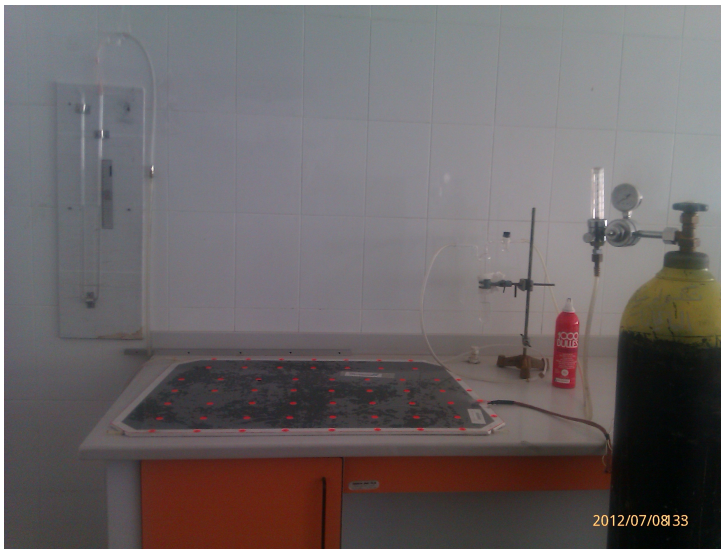
Figure 3.7: leak test system
