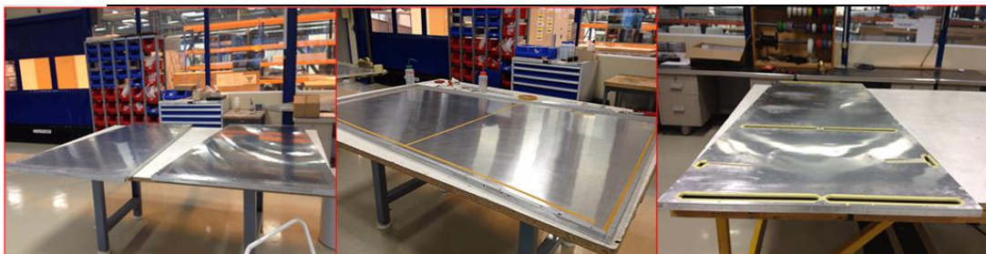
Figure 5.23: Mechanics preparation for chamber assembly – putting Mylar and insulation tape.
