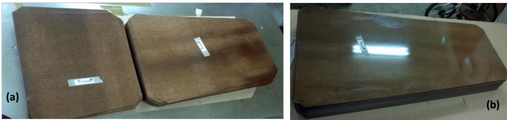
Figure 5.6: Bakelite sheets cut for the RE4/2 top narrow and top wide gaps (a) and bottom gaps (b).
