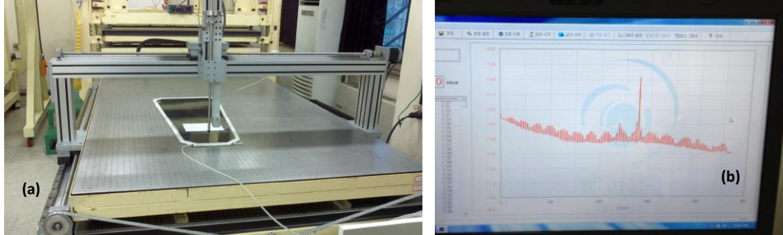
Figure 5.8: KODEL robot performing the pressure test (a) and the control console of the pressure test (b).
