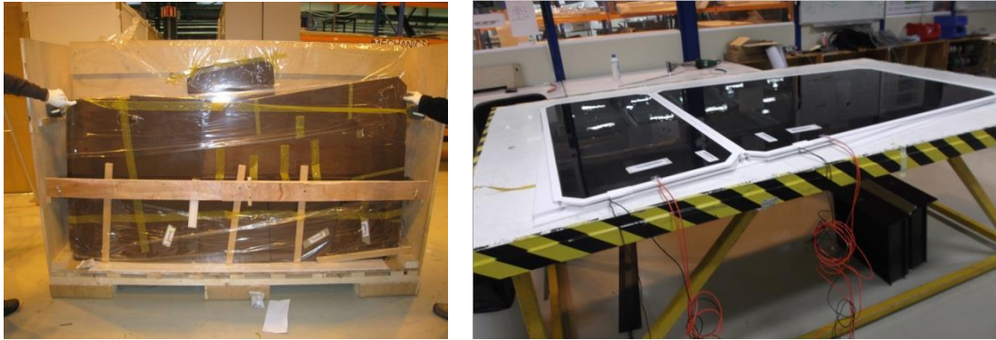
Figure 5.17: Taking the gas gaps out of the transportation boxes
