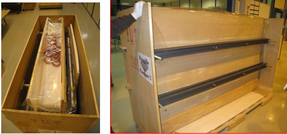
Figure 5.10: Specially designed wooden box for gaps transportation.
