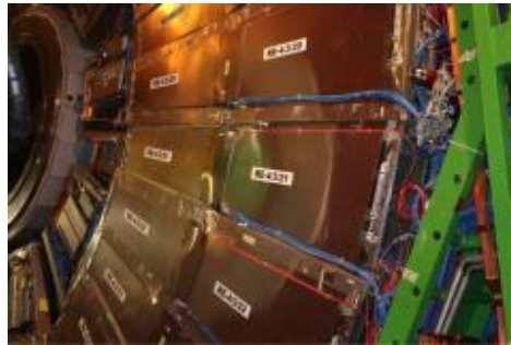
Figure 5.44: Zoom of the RE4 negative disk, covered with RPC detectors.
