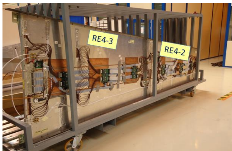
Figure 5.34: RE4 Super Module ready for installation on the CMS Endcap disks.
