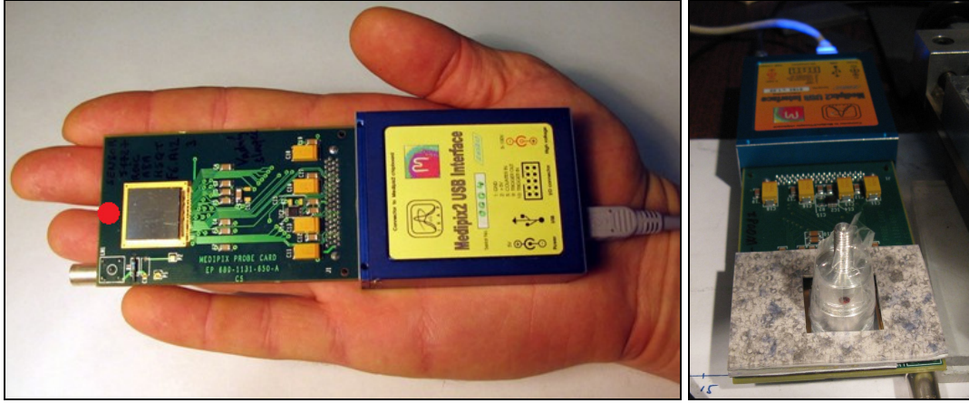
Fig. 24. View on the Timepix detector. Left: detector chip and chipboard with USB readout interface. Red dot on the left side marks the orientation of the solid sources during measurement, see text. Right: geometry of the measurement with source placed in the source holder and covered by a mylar foil.
