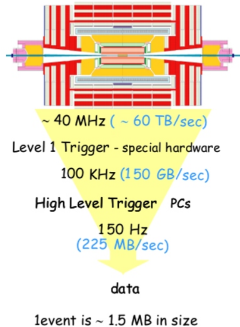
Figure 3.1: Overview of the CMS online trigger system with the corresponding trigger rate and data flow.
