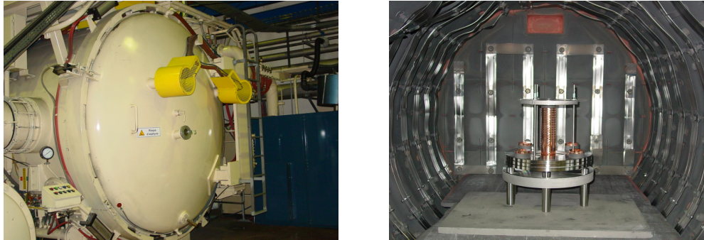
Figure 1.16. Outside and inside view of bonding oven [17]
