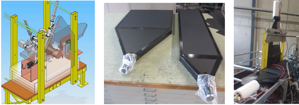
Figure 5.8: Schematic view of the muon vetos over the SSMM detectors (left) and photographs of the plastic scintillators on a test-bench (center) and installed in CAST (right).
