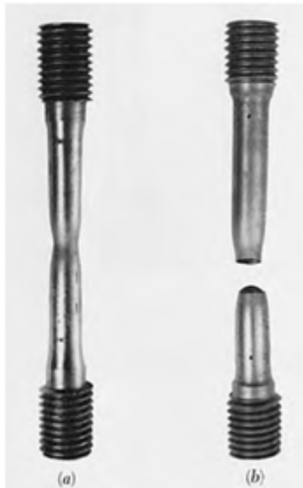
Figure 8. Necking (a) and final rupture (b) of a ductile test specimen.
