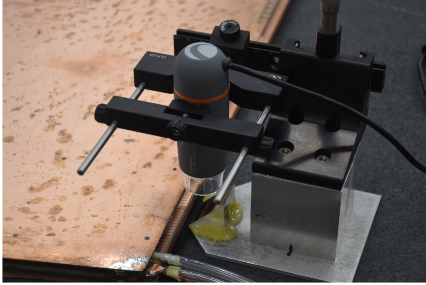
Figure 28: Microscope assembly used for measuring alignment of sTGC doublets and quadruplets.
