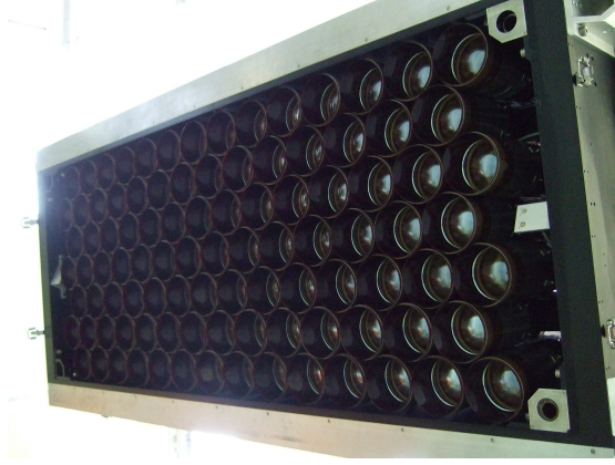
FIGURE 4.1: Upper HPD grid in RICH 1
