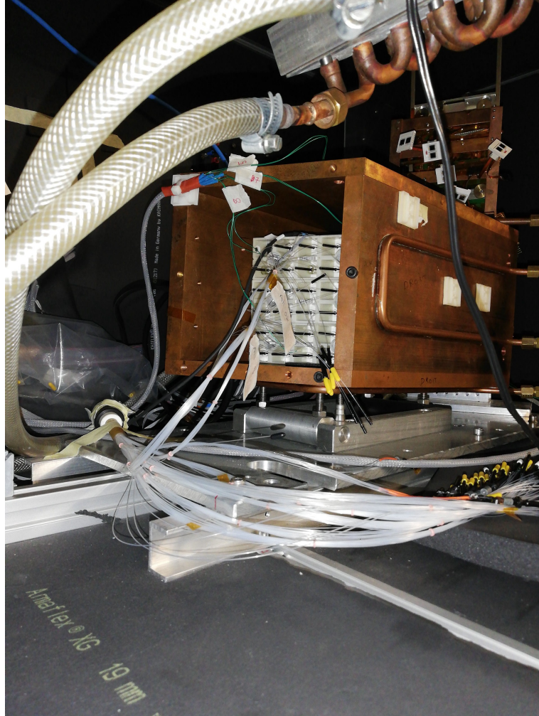
Figure 5.2: Inside the box used for the 2018 test beam run. The crystal matrix can be seen inside the copper coloured box, while there are bare APDs (i.e. not mounted to a lead tungstate crystal) above this. Though the crystal matrix itself is 5x6, only five of the six crystals per column could be read out as the VFE is limited to five channels. Photo provided by Simone Pigazzini.
