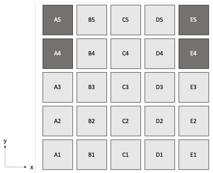
Figure 5.5: Matrix scheme of the lead tungstate crystals for the June 2018 test beam. The four dark grey crystals - A4, A5, E4 and E5 - did not collect data during this test beam run due to broken VFE adaptors. Each column refers to one VFE.
