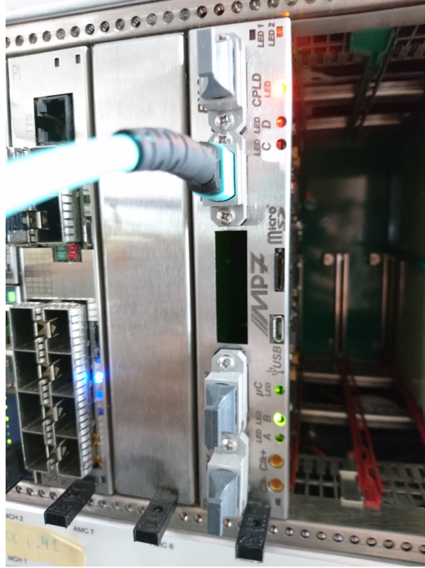
Figure 6.2: The MP7 board used for the hardware test of the LD algorithm and the later test of the combined Swiss-cross and clustering algorithm. The attached cable was irrelevant to the test described in this thesis as data was loaded and read out via the crate’s backplane.
