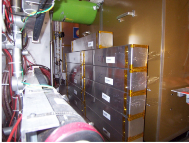
Figure 22: Left: Photograph of the 2012 MMT test array placed downstream of the LHCb stacked under the beam pipe 1.8 m away from the interaction point along the back of the VELO vacuum vessel.
