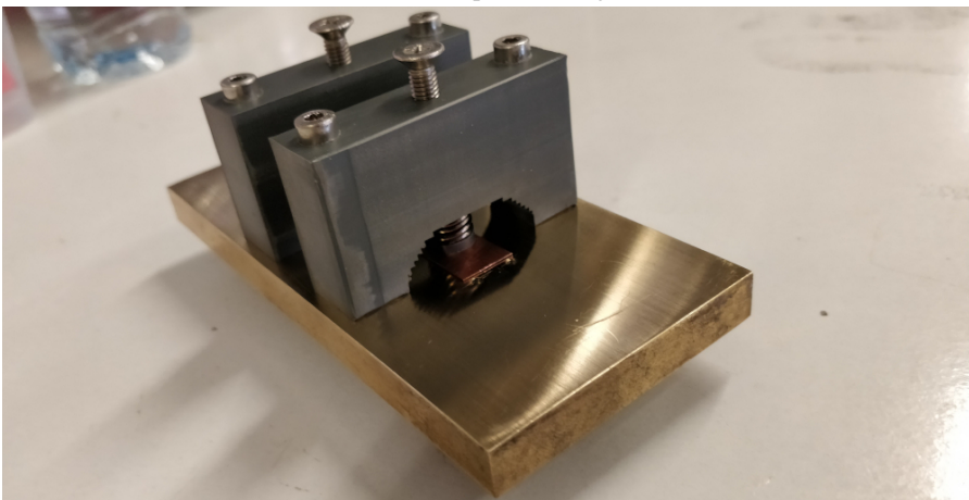
(c) 5 cm PPR with PVC bridges and screws
