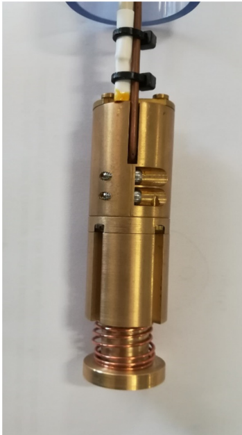
(b) Closed dielectric resonator with the positioning of the Cernox T -sensor at the top of the assembly and elongation piece at the bottom for conduction cooling.
