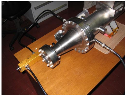
Fig. 4.53 Hybrid connection to the kicker end
