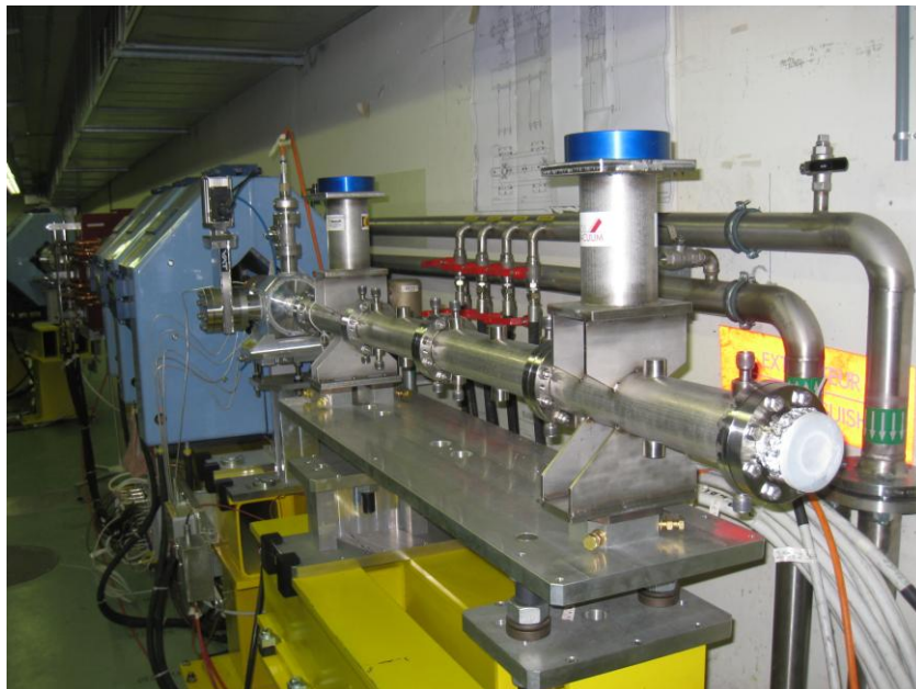
Fig. 5.47 Tail Clippers installed at CERN in CTF3 TL2 zone
