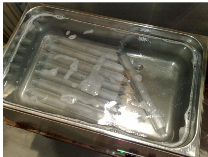
Fig. 5.30 Ultrasonic bath cleaning of Tail Clipper electrodes
