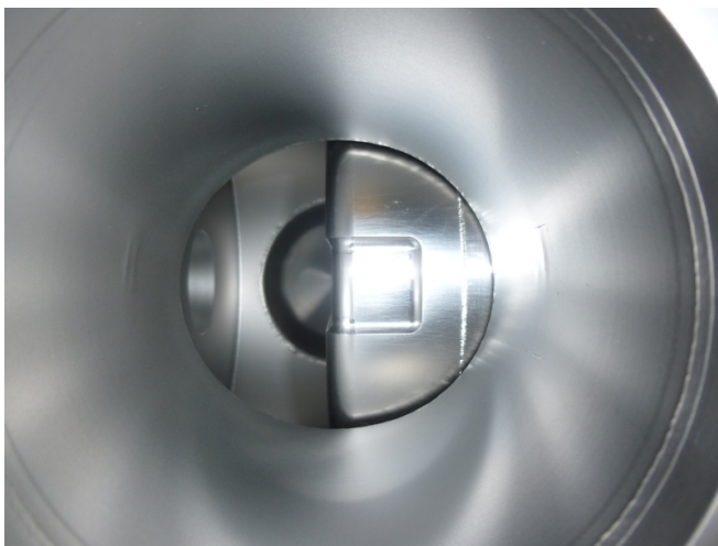
Figure 1.15: View of the Roman pot inserted in the beampipe [12].
