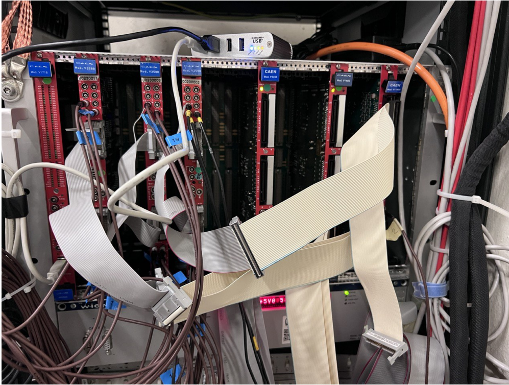
Figure 6.2.11: The Picture shows the VME-crate with the three discriminator on the left connected to the CAEN TDC on the right.
