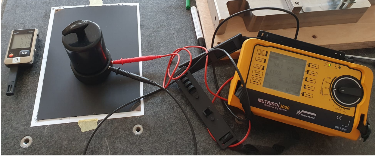
Figure 5.3.3: Measurement with of the surface resistivity of the graphite.
