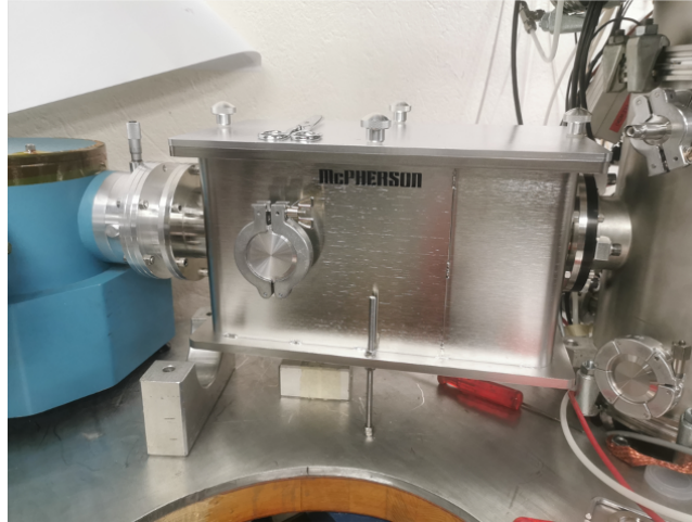
Figure 5.10: The collimating mirror chamber that replaced a simple collimating lens.
