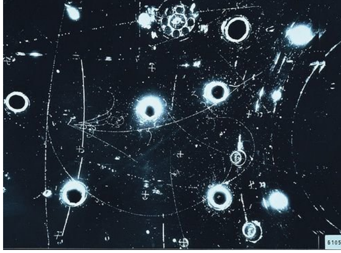
Figure 1.24: Example of a track from a neutral current interaction in the Gargamelle bubble chamber [102].
