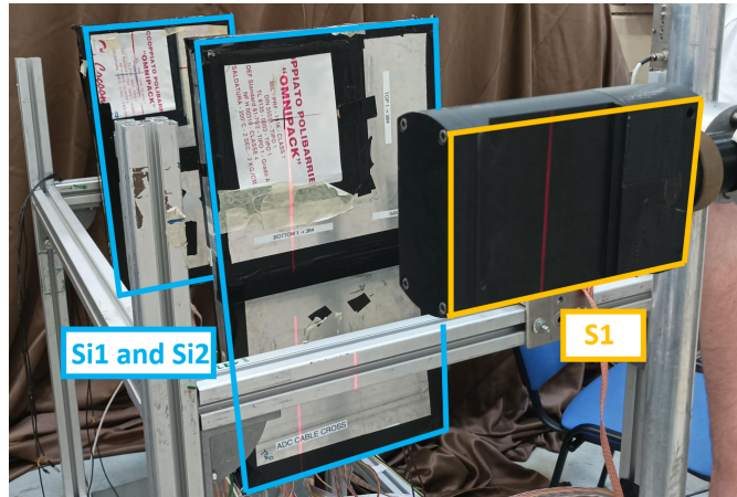
Figure 3.4: The S1 plastic trigger scintillator (orange) and the Si1 and Si2 silicon chambers (light blue). The red laser was used for the alignment of the system.
