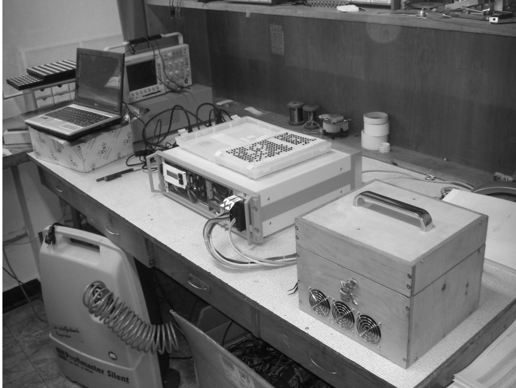
Figure 4.1: The complete device during normal operation. The feeder box (on the right) is connected to the electronics case (on the left) with a wiring harness. There is an opened pack of MPPCs on the top of the electronics box
