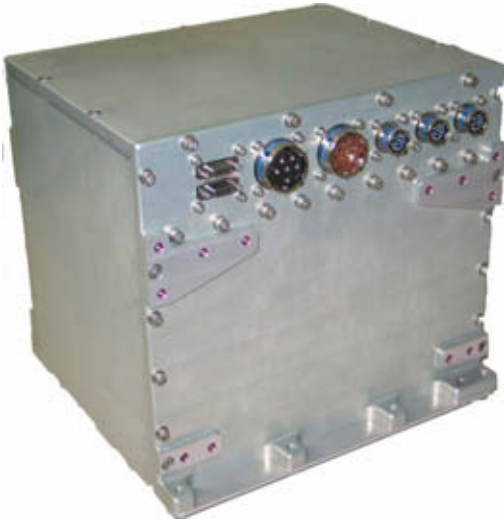
Figure 4.19: Photo of the UPD box. Visible is the right main wall with the 28 V supply and the HV as well as digital 3.3 V output connectors.
