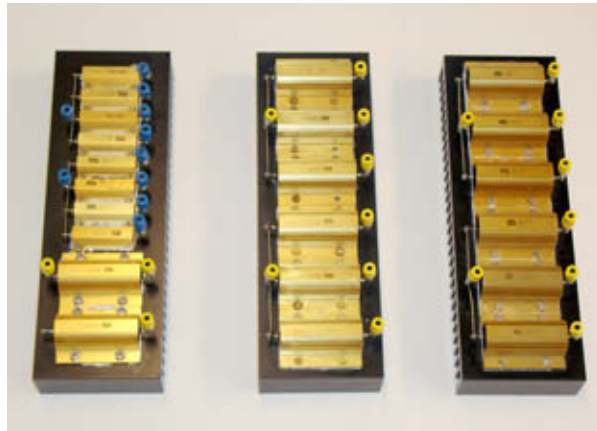
Figure 4.50: Photo of three resistor chains used for manual efficiency measurements of the DC/DC-converters.
