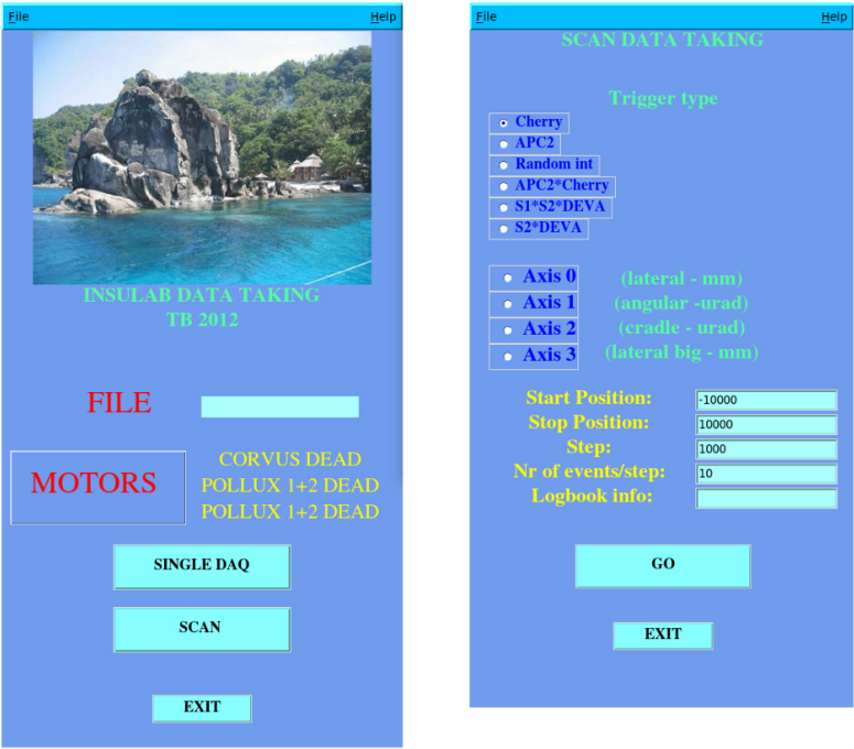
(a) Left panel: main software window. Right panel: data acquisition for the SCAN modality, where the trigger and the scan boundaries can be set.
