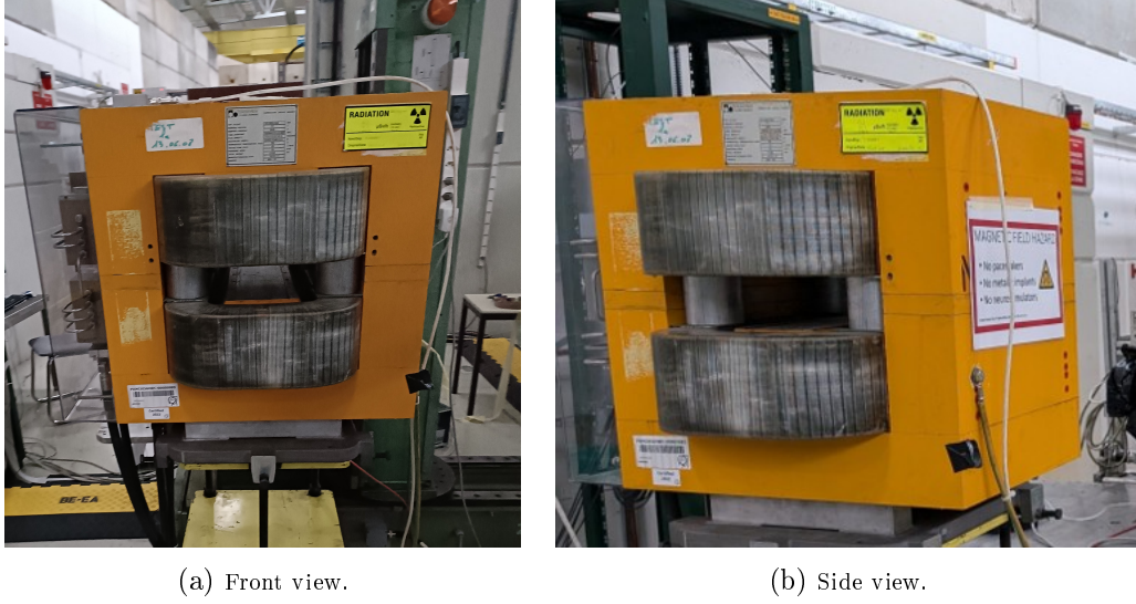
Figure 3.13: Front view (a) and side view (b) of the dipole magnet in the beamline, for the curvature of charged particles after the interactions with the crystalline radiators.
