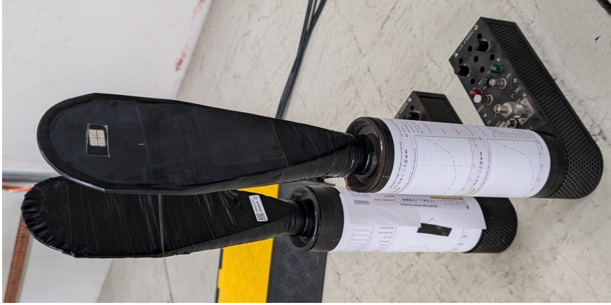
Figure 3.16: Photo of the scintillator modules used in the 2024 beamtest.
